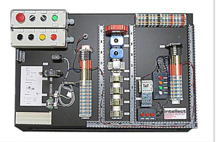
MC-100: AC and DC Variable Speed Motor Drives
